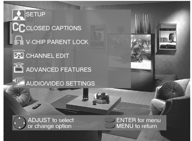
Figure 1. Main Menu: The Main Menu screen will always be the first screen that appears when you press the MENU button.
